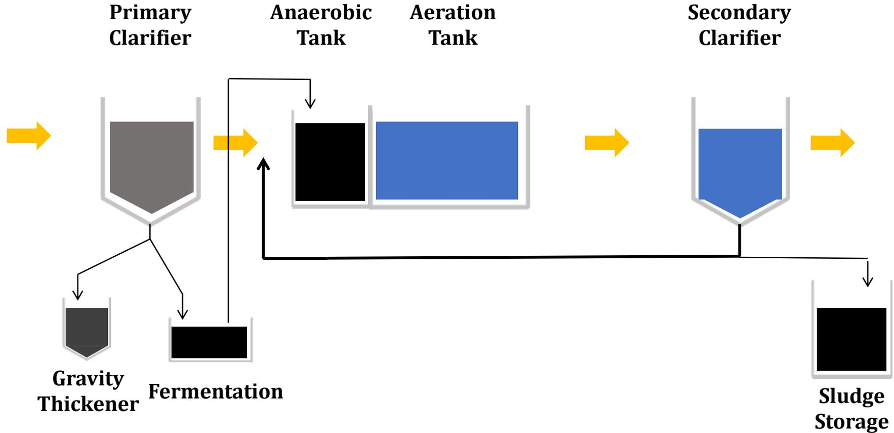
**If Anaerobic Tank isn't really anaerobic ...**
