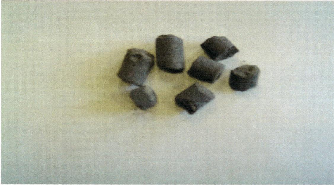
**Photograph 1: 12mm diameter Green Pellets (Commercial Flat Die Pelleting Press)**
