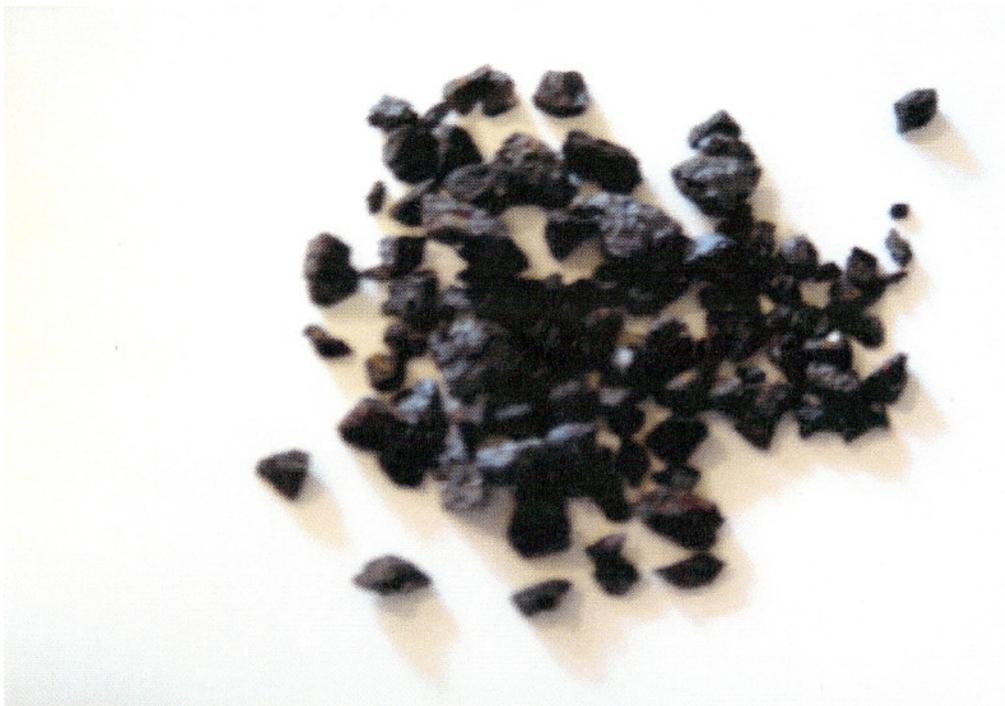
**Photograph 16: LWA Produced from fired briquettes after crushing and sizing**
